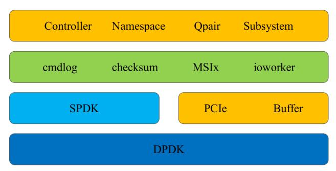
We then wrap all these SPDK and pynvme functions in a Python module. Users can use Python classes (e.g. Controller, Namespace, ...) to test NVMe devices. Here is an identical script as SPDK's 400-line example: https://github.com/spdk/spdk/blob/master/examples/nvme/hello\_world/hello\_world.c
